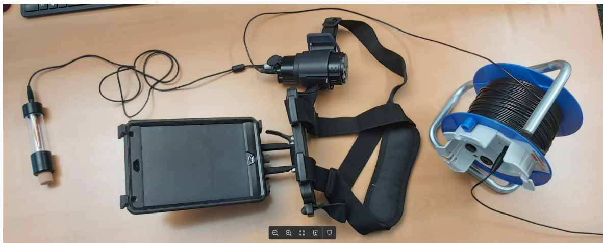
Figure 7 : PM8500 Rod electrode cabling set up
