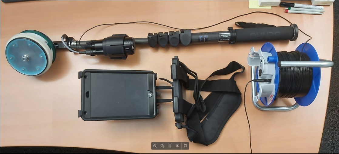
Figure 8 : PM8500 One wheel electrode cabling set up
